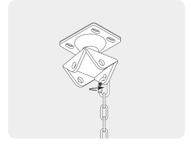
CAUTION: It is extremely important that you perform a monthly inspection of all swing type activities. The components MUST be checked for wear and to make sure all of the hardware is tight. The Tire Swing Hanger is also equipped with a grease fitting and should be lubricated periodically.
