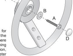
Step #2 Insert the 5/16 x 2" Lag Screw through the 5/16" Flat Washer and through the Steering Wheel as shown.
