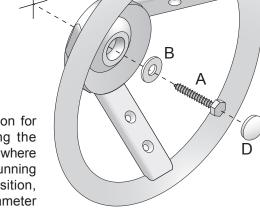
Step #2 Insert the 5/16 x 2" Lag Screw through the 5/16" Flat Washer and through the Steering Wheel as shown.
