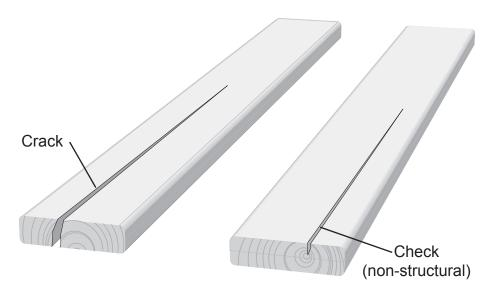
ture and moisture conditions. A check is not a crack – it does not affect the strength or durability of the part and is not covered under warranty. If you have ever noticed large beams in a barn or old building, you will see similar checks. Yet, many of these structures are still strong after dozens or even hundreds of years! You can slow (but not stop) the checking process by maintaining the water repellent finish on your set.
